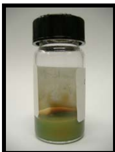
Figure 1. Microgels composed of NIPA monomer and functionalized CNTs. CNTs are encapsulated within the microgels.
